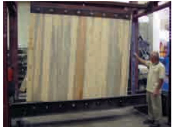
Figure 6: ICLT in-plane lateral load testing
